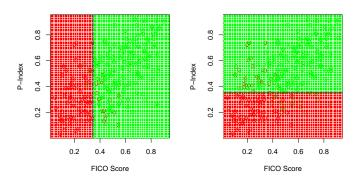
For the best cut on FICO Score there are 21 classification errors. For the best cut on P-index there are 47 classification errors. Therefore the first cut is on FICO score. By inspection one can see that the second cut will have to be on P-index.
